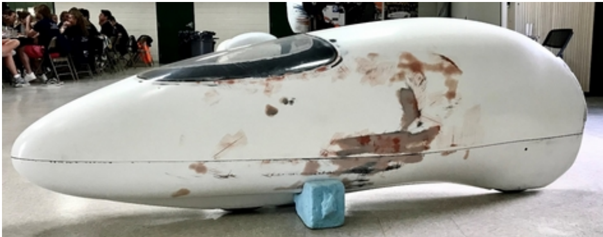
Velox XS after fixing the scratches of a crash at 113 km/h in Battle Mountain
