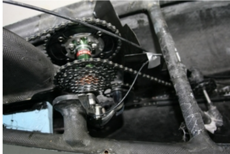
Rear wheel drive with intermediate gearing for reaching high speed.
